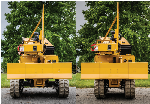
The expandable, non-marking rubber track undercarriage provides a stable, 50-inch wide, stance for cutting while retracting to 35-inches to squeeze through backyard gates.
