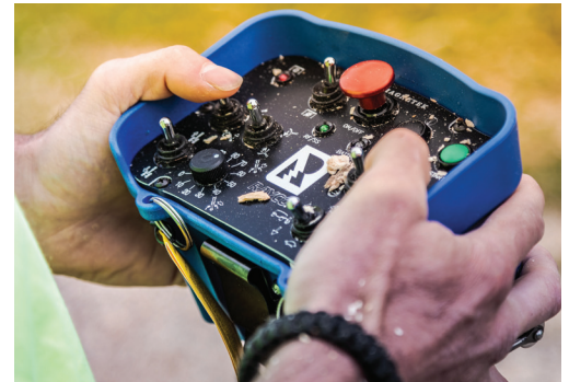
The wireless remote control unit is sealed against dust, water, and other elements.
