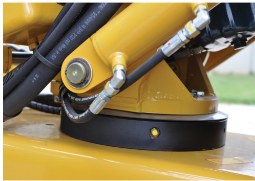
Slewing ring pivot on cutter head swing Maintains constant depth across entire Swing width.
