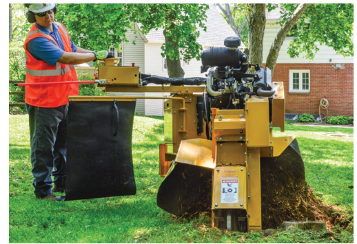
Swing-out chip retainer curtains keeps operator protected from debris.
