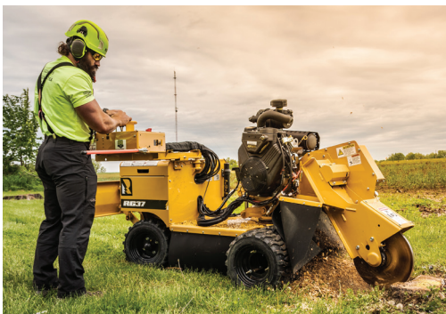
Swing out control station for better visibility. Controls fold in line for travel through gates.
