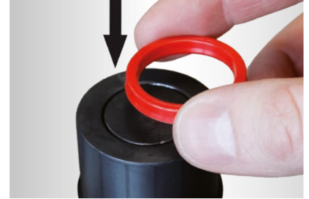
Press together new sealing washer and place on the sealing disc with the open end facing downwards.
