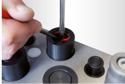
Press down sealing disc on the coupling plug with a screwdriver and remove the top sealing washer (red) with a sharp tool.
