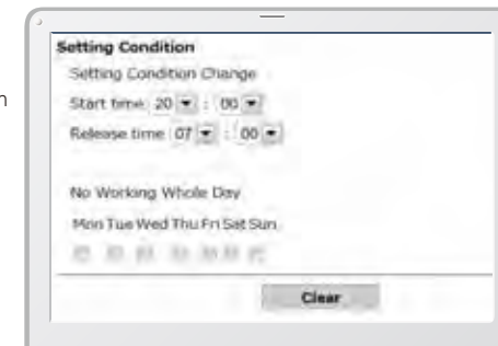
Engine start alarm outside prescribed work time
