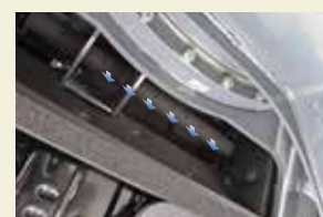
Holes on the muffler disperse exhaust
