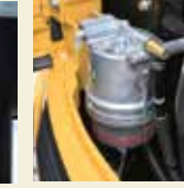
Pre fuel filter with built-in water separator
