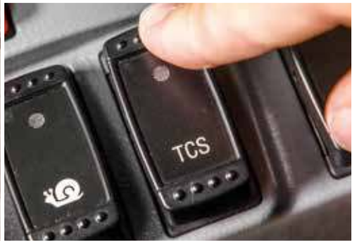
The traction control system reduces tire slippage in wet or wintry conditions.
