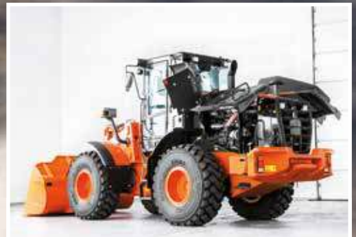
Easy access for maintenance from ground level.
