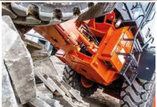
The optional belly guard provides added protection.
