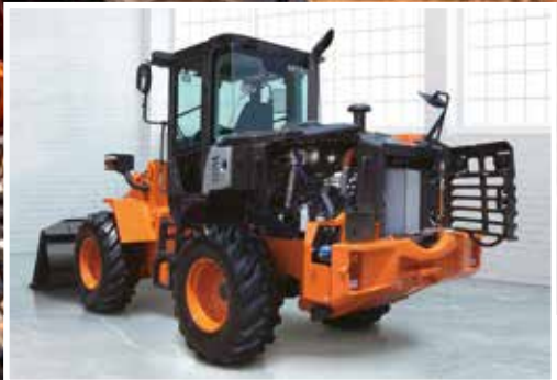
Easy access for maintenance from ground level.
