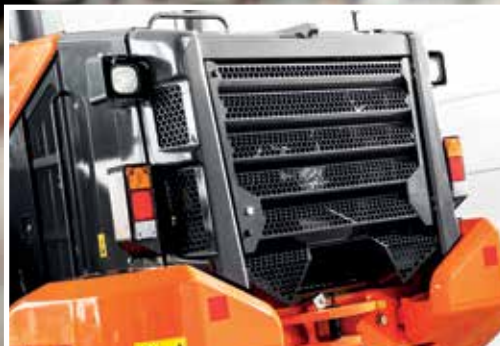
New rear grille protects radiator compartment.
